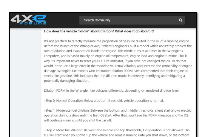
· Step 3: More fuel dilution: Above the top threshold, EV operation is not allowed, and the vehicle will
