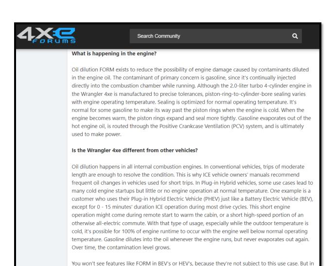
PHEVs from other manufacturers, you'll see warnings like "Low Engine Use Mode," "Maintaining Hybrid mode to protect engine," or "Engine Maintenance Mode," which all do the same thing as
