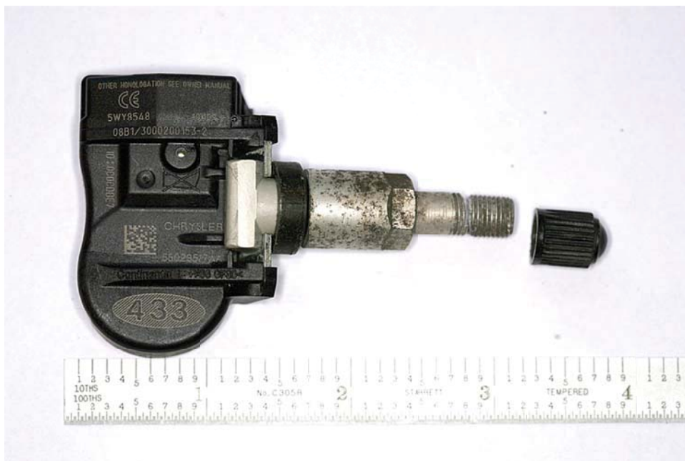
Figure 3-1 — TPMS Device Sample A with Fractured Stem.
