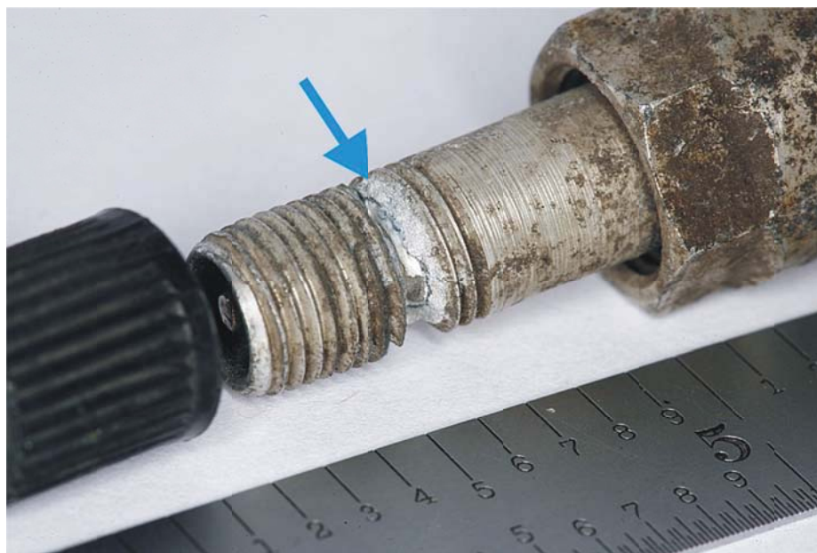
Figure 3-2 — TPMS Device Sample A, Close-up of Fracture (At Arrow).
